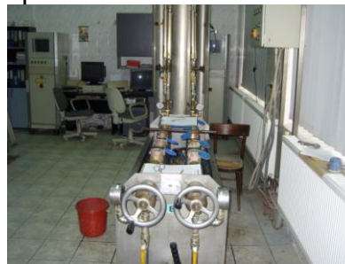
Figure 4. Metrological verification stand of water meters [1]
