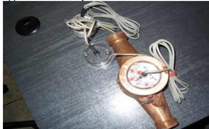
Figure 1 DN 32mm water meter equipped with REED relay data transmission [5]
